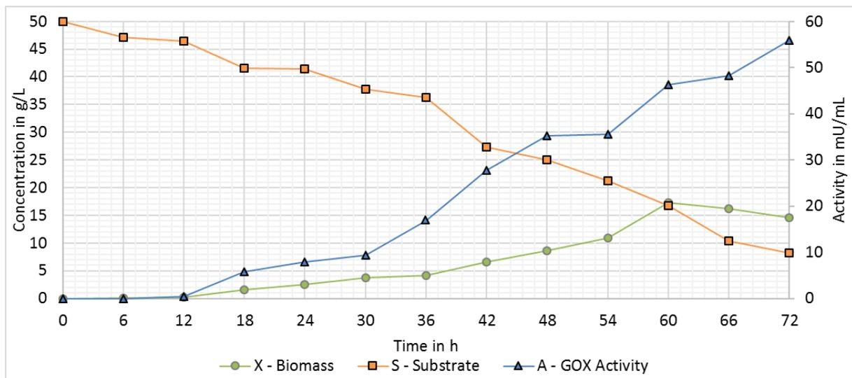
Figure 5.2: Small scale fermentation: 50 g/L glucose
