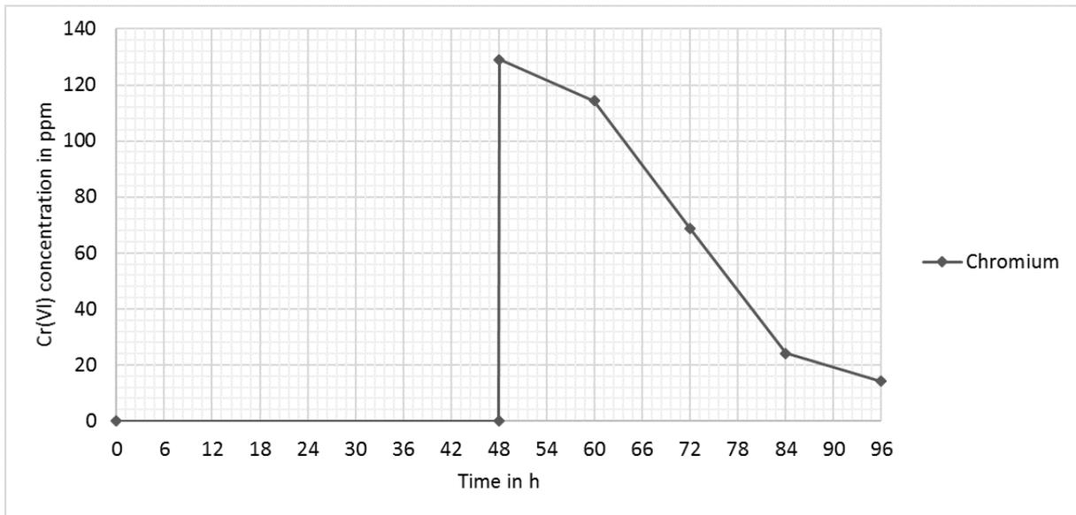
Figure 5.11: Stirred tank: Chromium reduction
