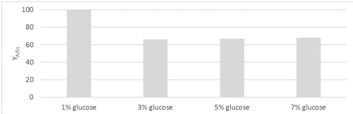
Figure 5.13: Stirred tank: Yield based on total substrate consumption (normalized)
