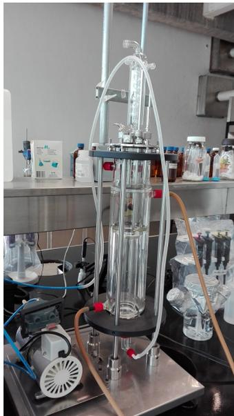
Figure 4.4: Airlift reactor
