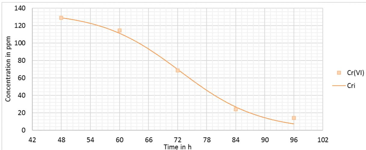
Figure 5.14: Stirred tank: Mathematical model of chromium reduction
