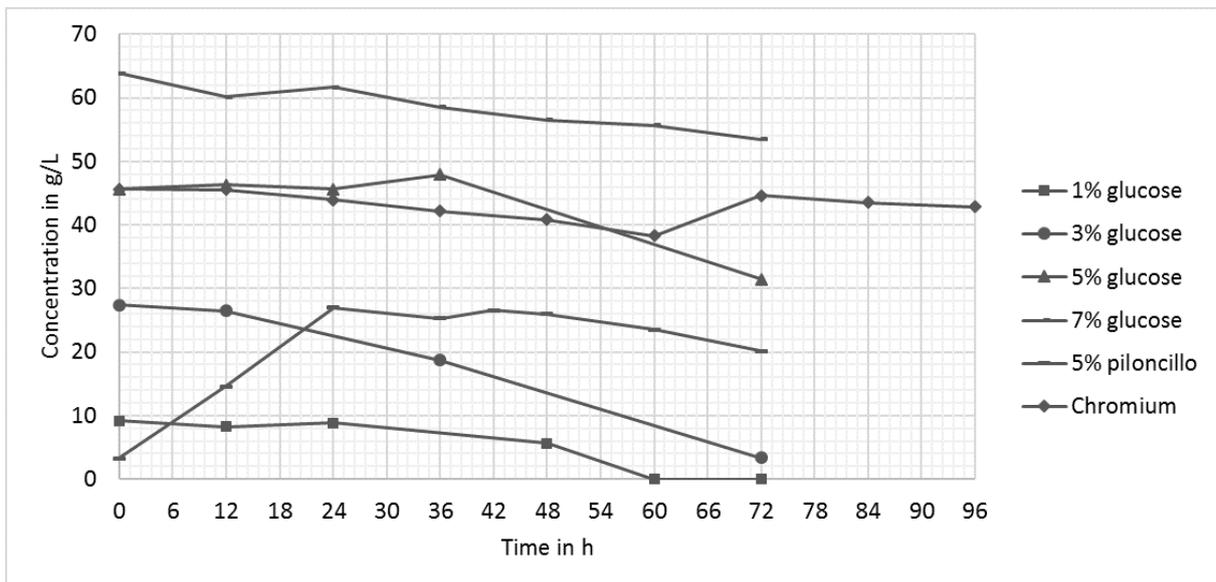
Figure 5.8: Stirred tank: Substrate
