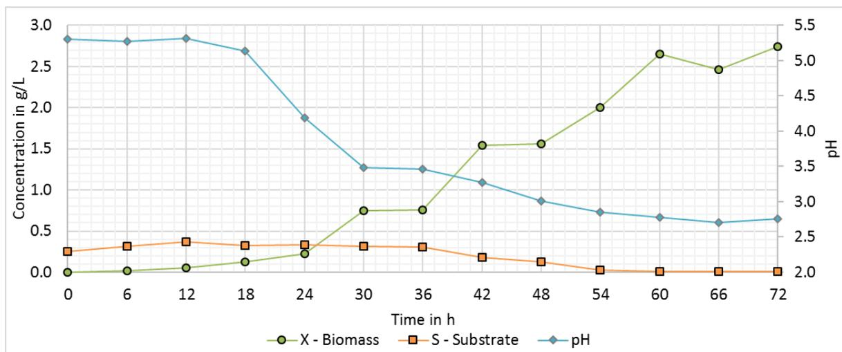
Figure 5.1: Small scale fermentation: 2.5 g/L glucose
