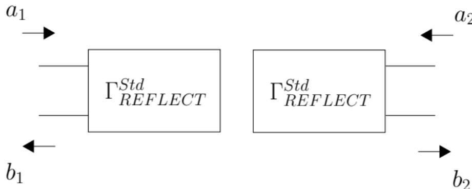
$$\Gamma_{REFLECT}^{Std} = \frac{b_1}{a_1} = \frac{\bar{T}_{21} + \bar{T}_{22} \cdot S_{11}^{Meas}}{\bar{T}_{11} + \bar{T}_{12} \cdot S_{11}^{Meas}} \quad (45)$$
