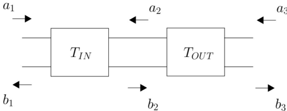
$$\begin{pmatrix} b_2 \\ a_2 \end{pmatrix} = \begin{bmatrix} \overline{T}_{11} & \overline{T}_{12} \\ \overline{T}_{21} & \overline{T}_{22} \end{bmatrix} \cdot \begin{pmatrix} a_1 \\ b_1 \end{pmatrix}$$
